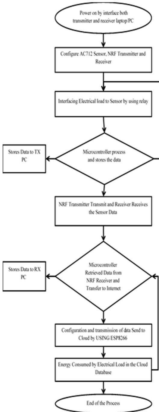
Fig. 2. Flow chart for basic mesh network
